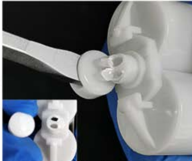
12. Wipe seal and keep in safe place for resealing if required.
