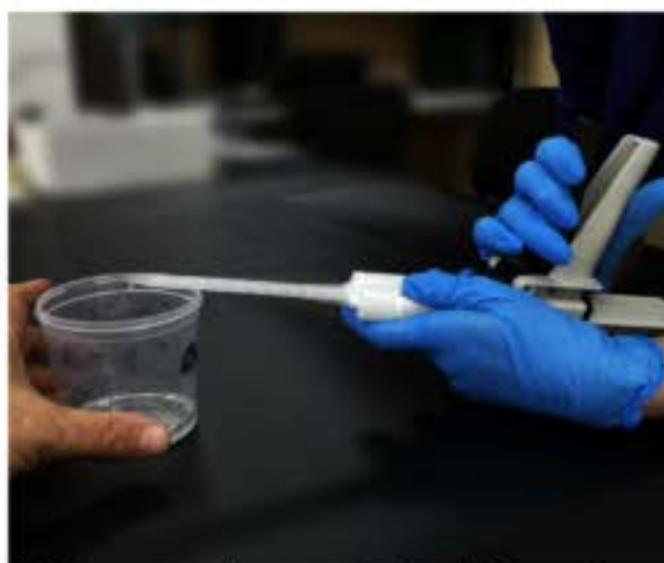
16. Purge small amount of resin from mixer to remove air. Incline gun and mixer to assist airflow.
