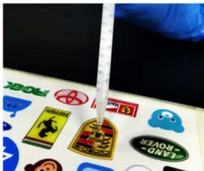
17. Apply resin, it will naturally flow to edge, too much and it will overflow, too little and it will be flat, practice is all it takes.
