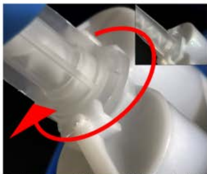
15. Turn mixer 90 degrees clockwise to lock into position.
