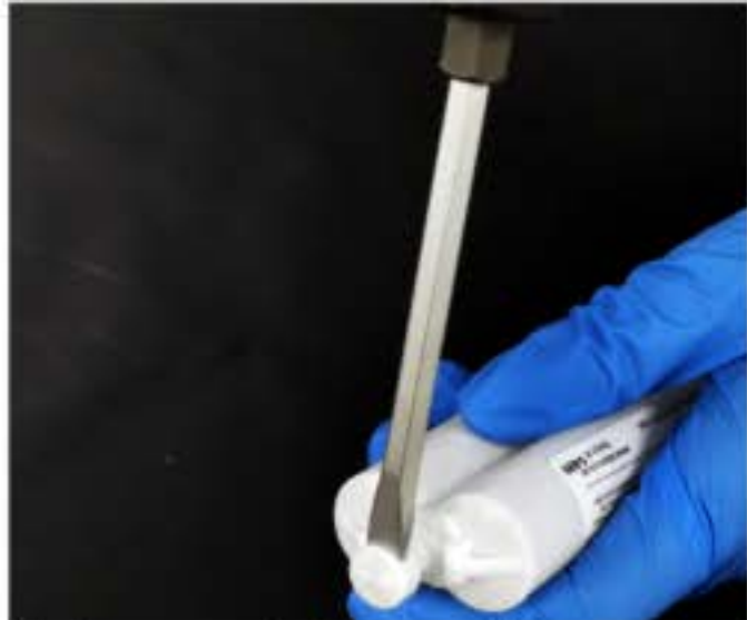
11. Remove seal using screwdriver.
