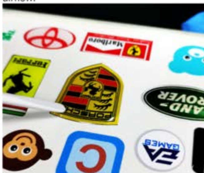
18. Difficult shapes might need assistance, use supplied plastic spatula to assist flow. Avoid sharp corners in your art work.
