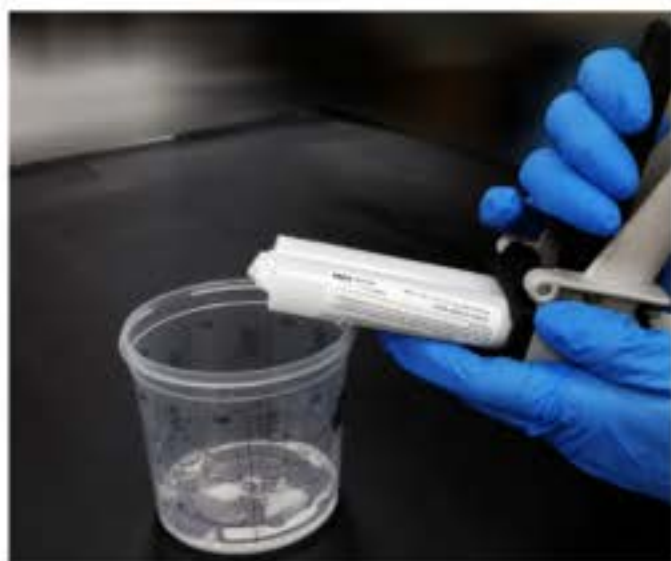
13. Purge cylinders until resin exits from both openings, inclining gun lower than receptacle.
